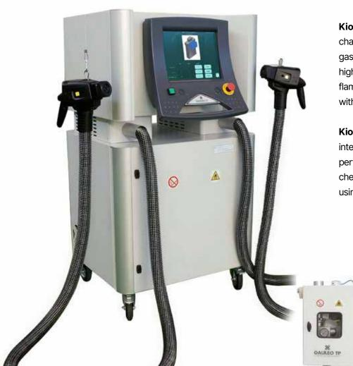
**Kion C** is the safest refrigerant charging system for flammable gases and is designed to support high production rates as well as both flammable and non-flammable gases within the HVAR industry.
