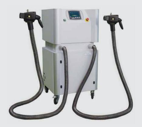
Agilis C is particularly indicated for small/medium production rates for both domestic and commercial refrigerators as well as freezers charged with non-flammables gases The machine automatically performs circuit evacuation, vacuum check, leak test and refrigerant charge using a self diagnostic system.
