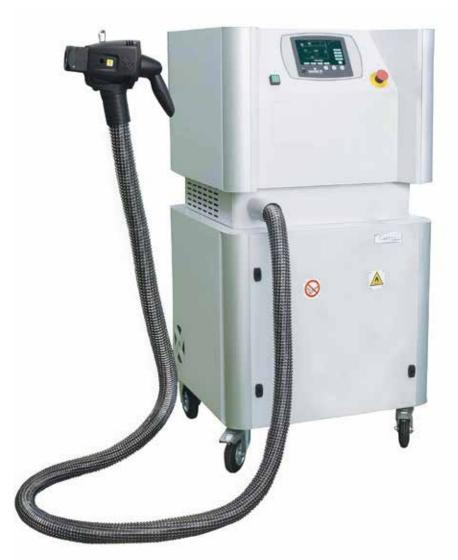
**Certus C,** a flexible and safe refrigerant charging system for both flammable and non-flammable gases in the HVACR market. Particularly suited for small/medium production rates. The machine utilizes a self-diagnostic system that automatically performs circuit evacuation, vacuum check, leak tests and refrigerant charge.
